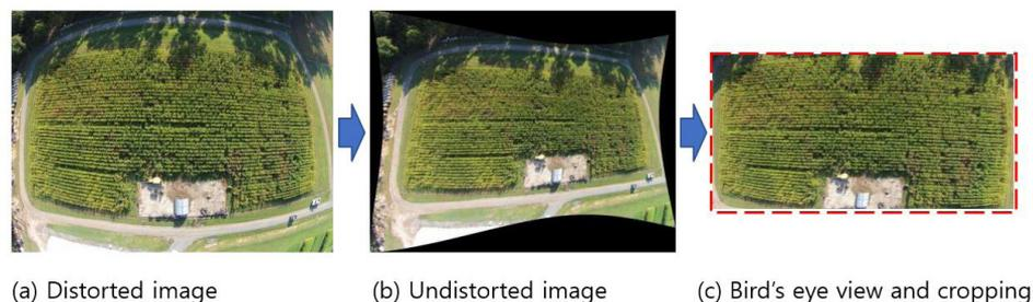
**Fig. 3.** Example of image correction.
