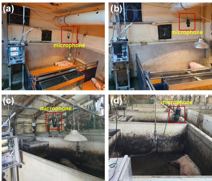
Fig. 2. Illustration of microphone positioning strategies in pig farm environments. (A,B) Microphone set up with additional sensors and data acquisition (DAQ) box for integrated monitoring, (C) microphone positioned at a moderate height above the pigs to capture ambient and individual vocalizations, and (D) microphone placed in close proximity to the pigs from above for an enhanced sound quality and specific behavior detection.
