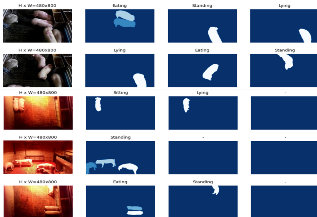
Fig. 7. Outputs of feature extraction for various pig postures using the improved algorithm. Each row represents different postures of piglets and pigs (sitting, lying, eating, and standing), with the extracted features highlighted in the corresponding columns. The size of each image is denoted as H \times W = 480 \times 800 , illustrating the segmentation results for each posture class.
